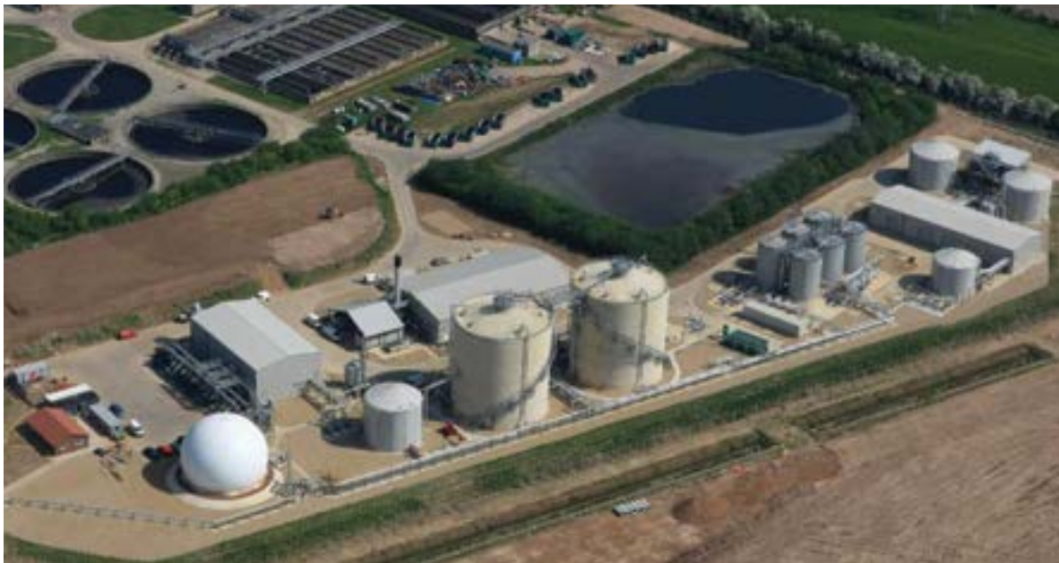
Biogas produced at the Anglian Water biosolids treatment facility in King's Lynn is used to generate heat and power for the entire wastewater treatment plant with the surplus exported to the national grid.
